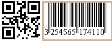
Figure 1: QR Code (2D) and EAN-13 (1D) barcodes encoding the same data (3254565174110).
